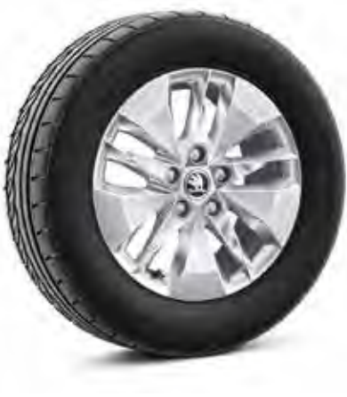
Kola z lehké slitiny TWISTER Aero, 16" (disk: 7J × 16" ET46, pneu: 205/60 R16)
